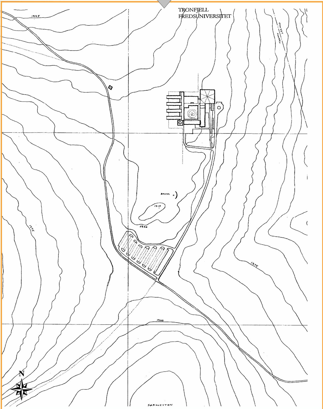
Site plan over the University of Peace at the 'Peace Plateau' on Mt.Tron. Here the car-parking and the road into the construction is seen. Between the car-parking and the university the memorial (menhir) is seen.
